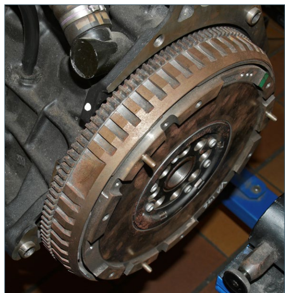
Picture 3: Encoder wheel on the flywheel of a Peugeot engine (DW10) // Photo: Guenther
