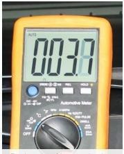
Resistance of heater circuit
