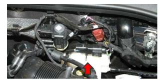
The connector is located in the engine bay, left
