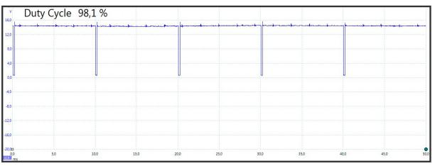
Duty cycle and frequency characteristic of heater circuit
