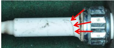
(disassembled spark plug- thread removed) Crack in the insulator portion, causing sparkthrough
