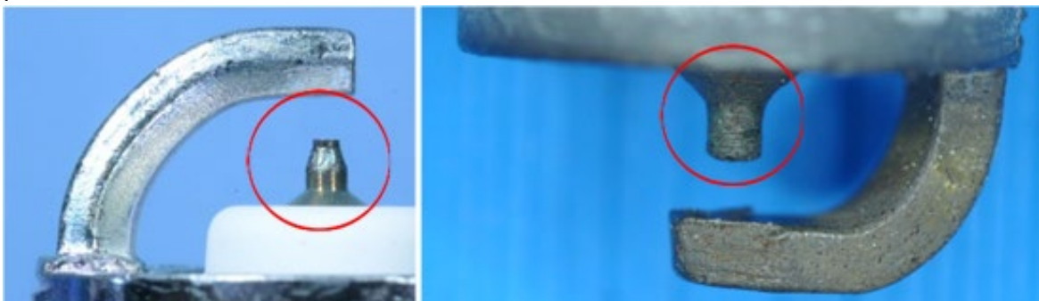
Left image: Electrode on an original product. Right: Electrode of a fake product.
