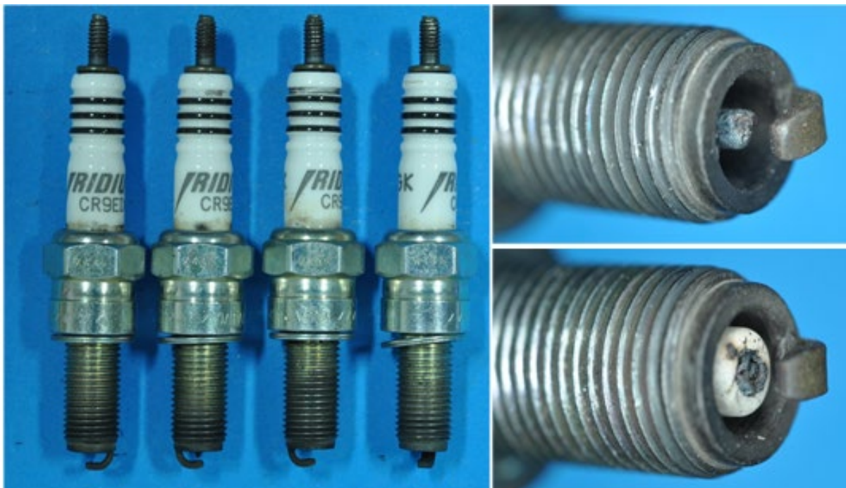
Examples of melted centre electrodes on fake CR9EIX spark plugs.
