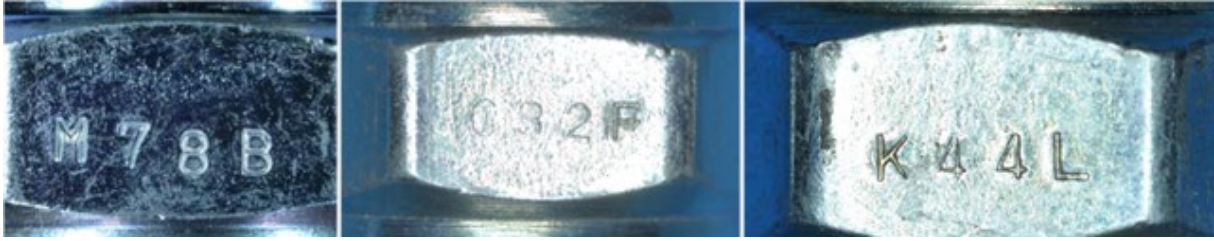
Left image: Original product with Lot Number and correct font. Both images on the right: Counterfeit products.
