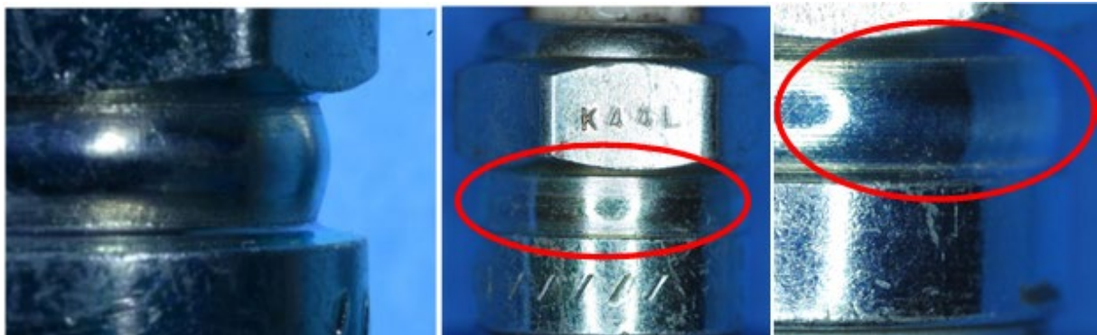
Left image: Original product without machine mark. Right: Machine mark from cutting on the surface of the metal shell on the C-Groove portion (counterfeit).
